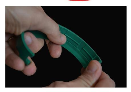
4. Push to join the two scraper's extremities. While contacting the extremities, slide down from the upper hole the included cotter pin (top-down).
