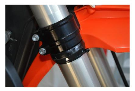
3. Clean area and install SKF Mud Scraper over the cave on the outer tube. Check mud scraper is positioned in its topmost position and seats correctly in the tube's seat. Check the scraping lip is contacting the chromed tube.
