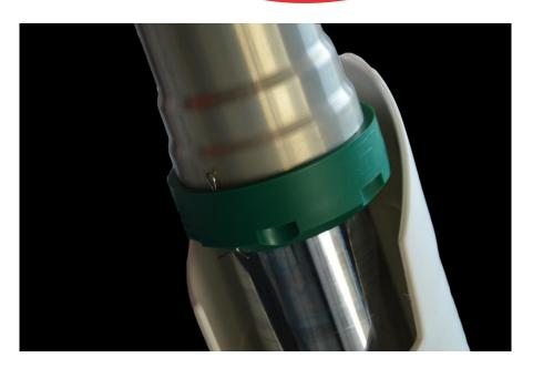
Check Mud scraper is positioned correctly and does not interfere with hole shot devices or other areas of the fork plastic shield.
