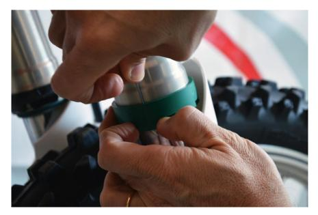
5. Release pressure and bend aside the two extremities of the cotter pin. Rotate the mud scraper to keep the cotter pin in the backwards portion of the tube.
