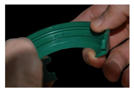
2. Clean area and install SKF Mud Scraper over the wear ring. At this stage you can repeat steps from point 4 as per WP installation steps.
