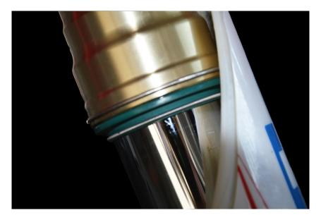
STEEL RING APPLICABLE MUD SCRAPER: please note the cavities that will have to be positioned over the OEM steel wear ring. Product presents two cavities at different heights to match position of the steel wear ring which may vary among fork models.
