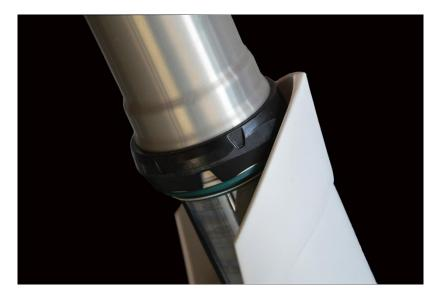
2. Once released you can slide the OEM plastic wear ring up over the fork until contacting the lower triple clamp. Lock in this position applying a plastic zip tie immediately underneath. Alternatively you can permanently remove the plastic wear ring, but in this case you'll have to remove the fork from the triple clamp.
